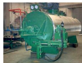
The cooker is equipped with a safety system for checking the opening of hatchways. If there is pressure inside the machine, the safety pressure switch don't consent to open the machine.
